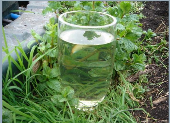
Effluent sample from a BioCube sewage treatment plant
